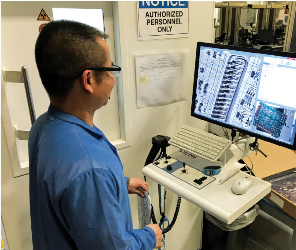
Namanh Phan, process engineer, uses the automated optical inspector (AOI) to look inside electrical components and check soldering joints on ball grid arrays. Photo by Mark Langlois.
